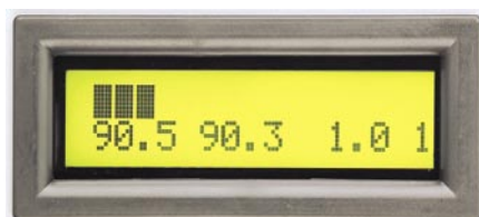
Figure 7 — The WN-2's numerical readout shows peak power, average power, SWR and sensor (up to four sensors can be connected at one time), as well as a bargraph for power output.
