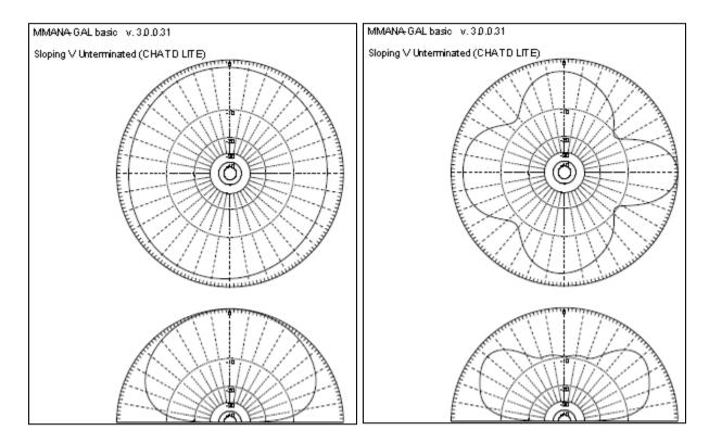
Figure 7. Sloping "V" Far Field Plots, 7 (left) and 21 (right) MHz.
