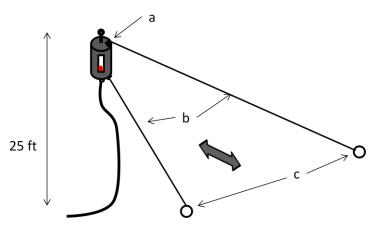
Figure 1. Sloping V Antenna Configuration.
