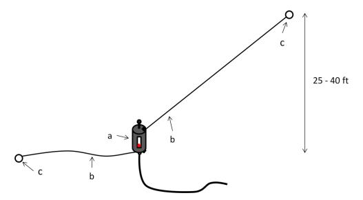
Figure 4. Sloping Wire Configuration.
