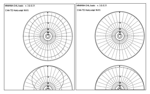
Figure 11. Horizontal NVIS Far Field Plots, 3.7 (left) and 7 (right) MHz.
