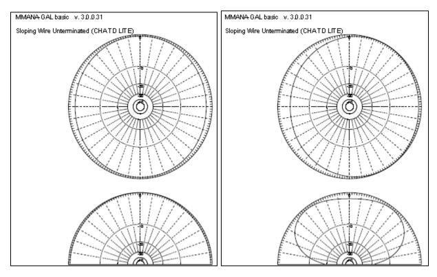
Figure 9. Sloping Wire Far Field Plots, 7 (left) and 14 (right) MHz.
