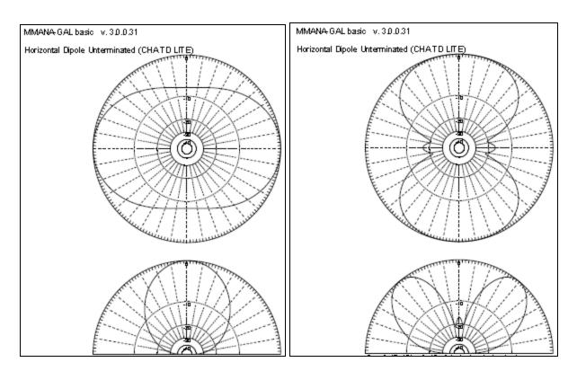
Figure 8. Horizontal; Dipole Far Field Plots, 7 (left) and 14 (right) MHz.
