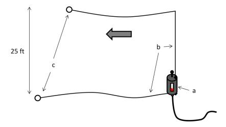
Figure 5. Inverted L Configuration.
