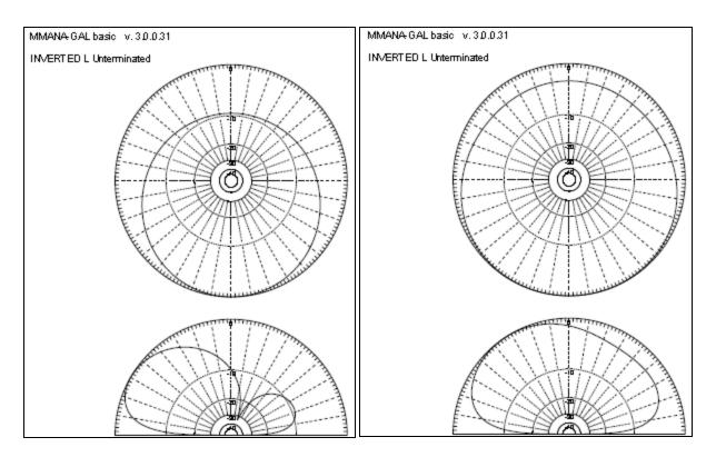
Figure 10 Inverted "L" Far Field Plots, 3.7 (left) and 7 (right) MHz.
