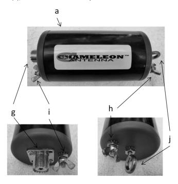
Plate 2. Matching Transformer, Side View (top), Bottom View (left) and Top View (right).
