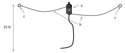
Figure 3. Horizontal Dipole Configuration.
