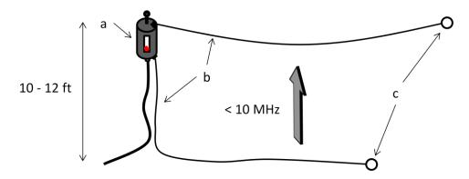
Figure 6. Horizontal NVIS Configuration.
