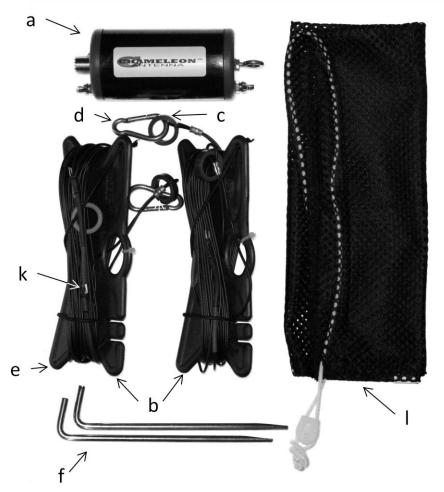
Plate 1. Tactical Dipole LITE Components.
