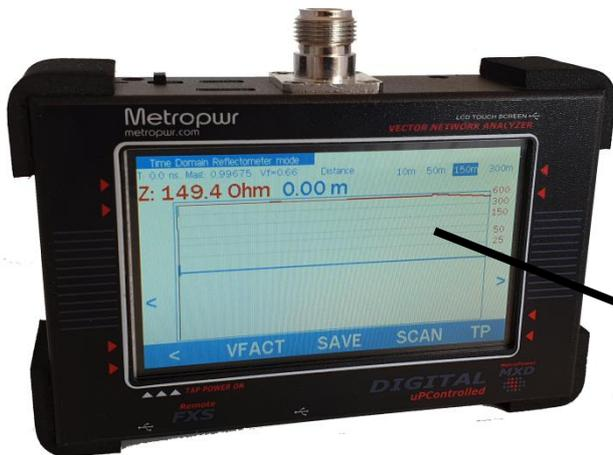
Menu for measuring the length of coaxial cables. It is possible to **select the velocity factor** for many types of cable. Selecting SCAN shows the graph and cable length. Cable failure is also possible here.
