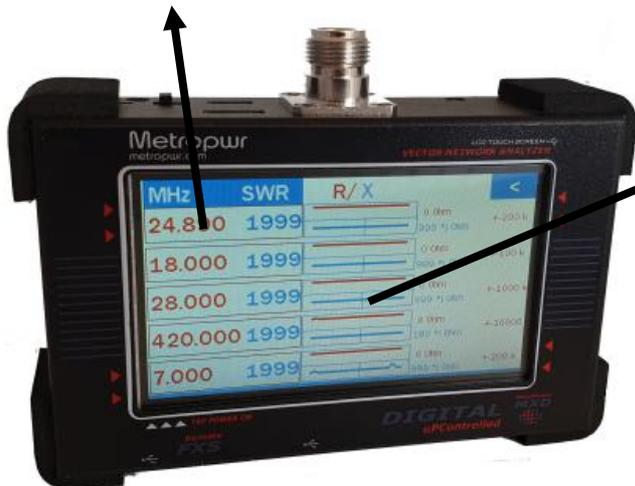
FX700/FX1300 can simultaneously measure SWR/R/X on 5 bands. This function is very useful for measuring multiband antennas.
