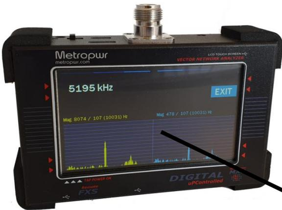
This is a service menu that displays the spectrum of V / I (voltage/current) signals taken from the measurement coupler.
