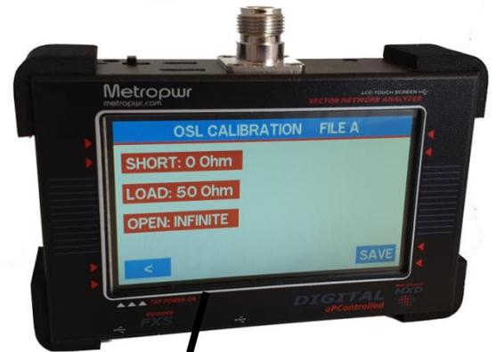
The calibration is necessary to compensate the cables connected on the DUT, this moves the reference plane to the end of the cable. Proceed with calibration by connecting in sequence SHORT/LOAD(50ohm)/OPEN tool and then SAVE calibration.
