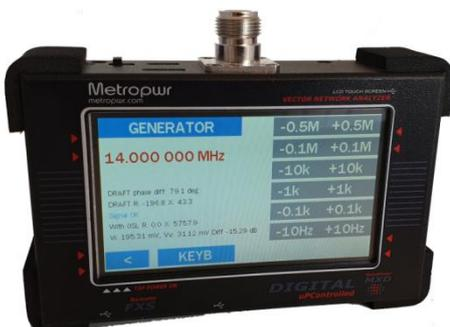
Menu Generator: possibility to select the frequency and set steps. A square wave and all harmonic frequencies will be generated on the DUT connector, no filtering expected.
