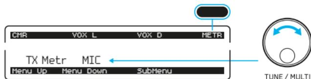
While speaking into the mic, adjust **MENU** → 09 > Gain > MIC (mic gain).
