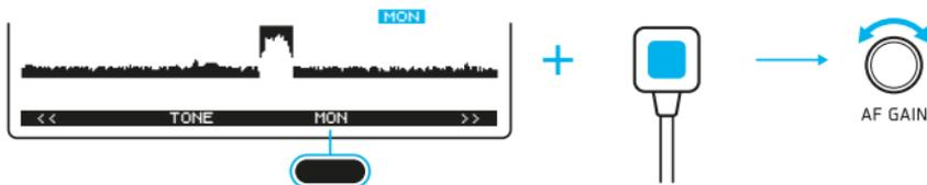
**!** Do not use the hand speaker-mic at the same time as monitor **MON** function in voice modes (**USB LSB AM FM**) – there is a risk of audio coupling with a high noise distorting the real audio.
