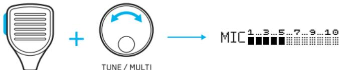
While speaking, adjust mic gain for maximum 5-7 bars on a scale. Mic gain for the TX-500 mic is typically 3-7.
