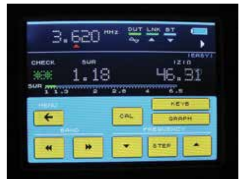
PHOTO 4: A good SWR at 3620kHz.
