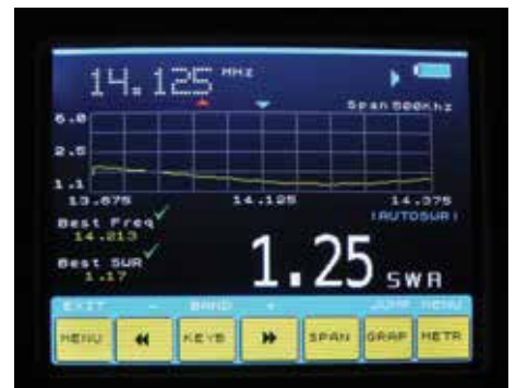
PHOTO 6: The AutoSWR screen for a 20m dipole.
