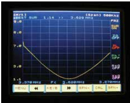
PHOTO 10: A good SWR dip on an 80m dipole.
