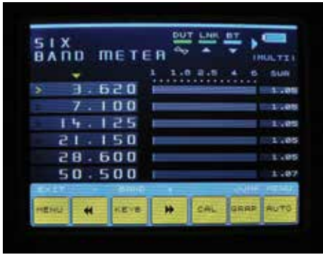
PHOTO 8: SWR across the HF bands of a 50-ohm dummy load.
