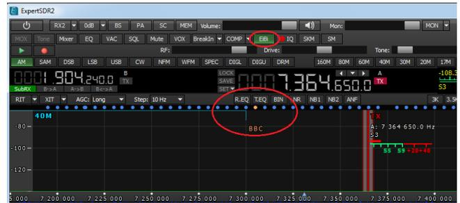
**IQ** - recording the IQ receiving channel on/off. The recording band is equal to the band displayed on the panadapter. The file is saved to the folder "C:\Users\User\ExpertSDR2\wave".
