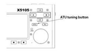
In actual operation, if the [HI-SWR] icon flashes on the screen, the tuning fails, and the SWR is large and needs to be tuned again.
