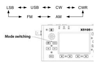
\*VFO-A and VFO-B can be set to different operating modes in the same frequency band, thus realizing the different operation modes of "voice /CW".
