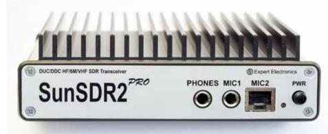
PHOTO 1: SunSDR2 PRO - front panel connections.
